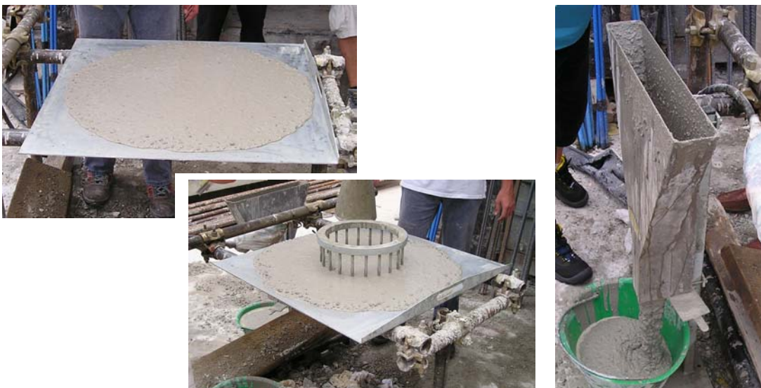
Fig. 4, 5, 6 - slump-flow, j-ring, V-funnel test.
